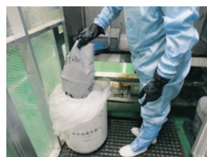
(5) Disposal of leaked substance
